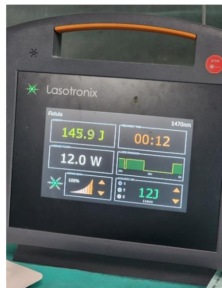
Figure 1: Lasotronix 1470nm diode laser machine, set at 12J with energy of 100-120 J/cm.
