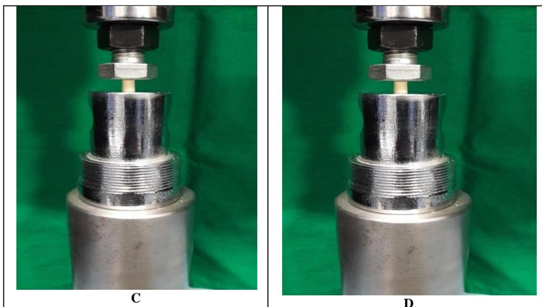
**Fig 11 – Apparatus for testing compressive fatigue strength of each cylindrical materials using universal testing machine A) Short fiber reinforced composite B) Amalgam C) Resin modified GIC D) zirconomer**
