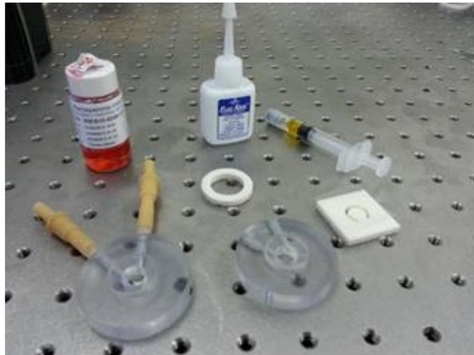
**Figure 1 Two polycarbonate discs with optical windows. One has two tubing connected for building up differential pressures and accurate measurements**
